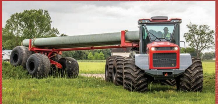
Designed for safe and efficient hauling of pipe, the ARDCO® AMT 600 Pipe Trailer offers adjustable lengths and up to 50,000 pounds of load capacity. Built to protect against pipe damage and featuring a flexible load rear frame, the Pipe Trailer is ideal for off-road transport in pipeline or utility construction applications.
