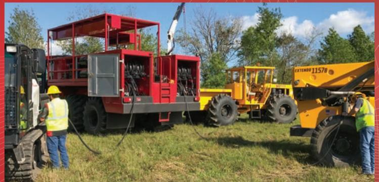
The ARDCO® AMT 600 Service and Lube Station includes a wide array of product delivery systems, including tanks for diesel, oil, coolant, grease and e-vac. Featuring a steel-constructed body platform with sheet metal roof structure, the station also includes ancillary equipment such as an air compressor, pressure washer, welder and crane.
